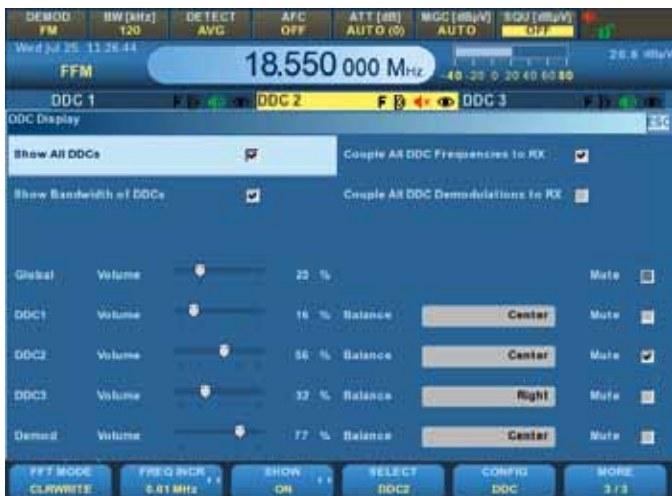
Control interface for managing of DDC information output.
