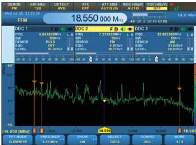
Smooth one plus three demodulation channels can be user-distributed within the realtime bandwidth.
